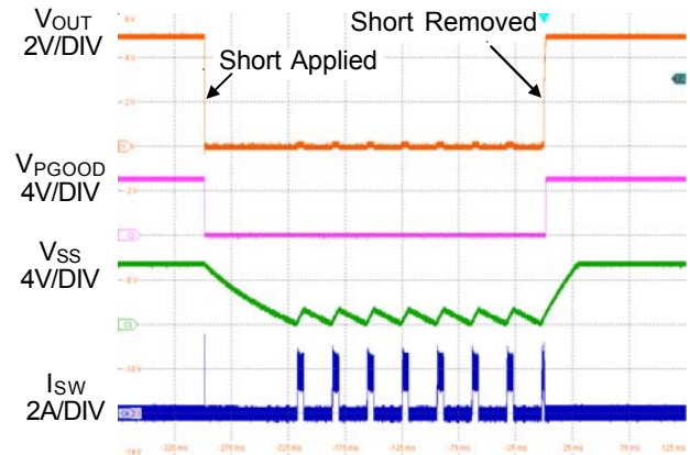
Figure 3. Short-Circuit Protection and Recovery
